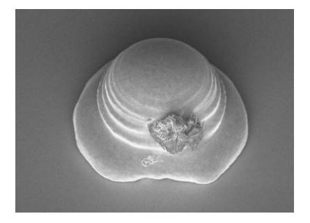
**Caption:** A laser pulse melted a tiny piece of metal on a silicon chip, resulting in an unexpected shape that looks like a very, very small Easter bonnet. An unintended dust particle serves as a decorative flower on its top. The size of the bonnet in this photo, measured from left to right, is about 45 micrometers, half the diameter of a human hair.
